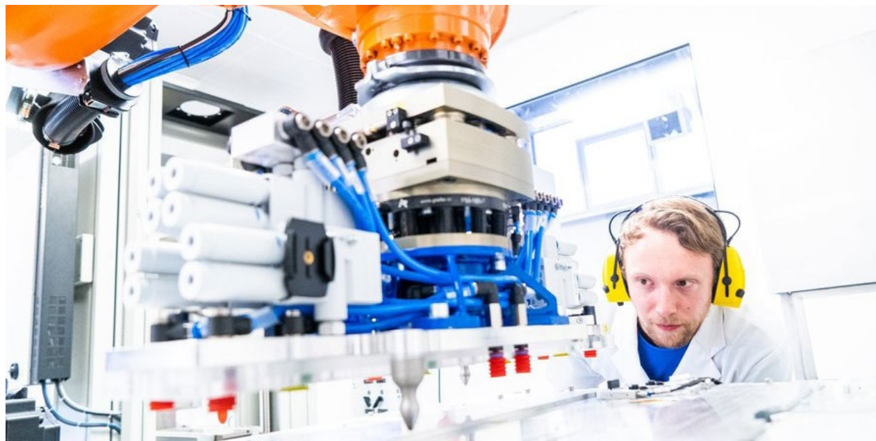
Robot-assisted fuel cell stack assembly.
