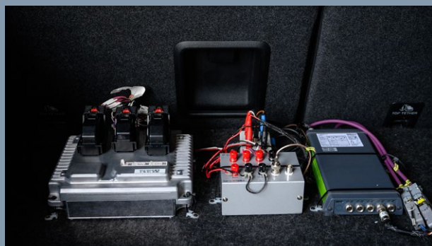
The DME injection system is operated by a control unit in the trunk. Engine and injection control communicate with each other via a specific CAN interface.
