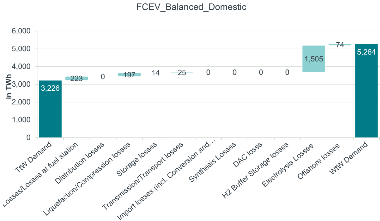
Figure 32: Energy demand along the domestic FCEV fuel supply chain [Source: Frontier Economics].
