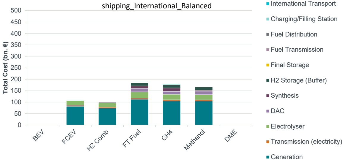
Figure 129: Fuel Supply Chain costs for shipping in 2050 exemplary for the international balanced scenario.
