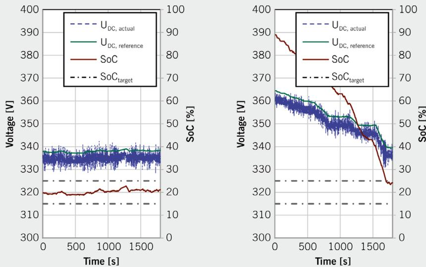
**FIGURE 4** DC link voltage and SoC of the battery as a function of the start SoC and the operating mode in CS mode (left) and in CD mode (right) (© KIT)
