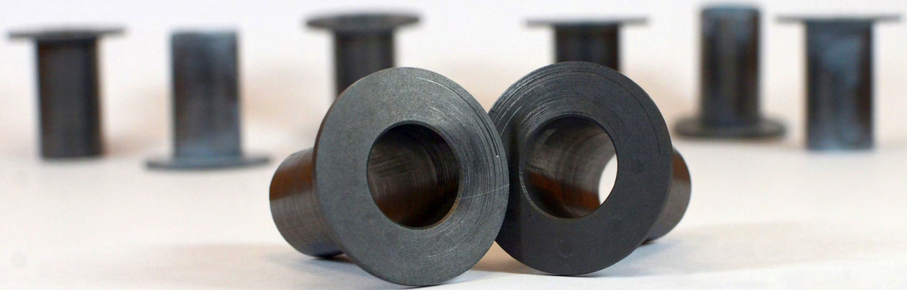
FIGURE 6 Prototype flange sleeves made of graphite infiltrated with aluminium or magnesium // TU Dresden | ILK
